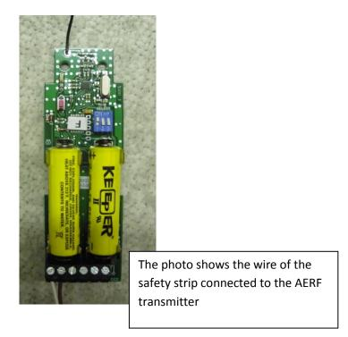
The dip switch of the transmitter has to be changed to the follow position:
