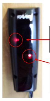
The upper LED is ON, the signal from transmitter will received, system is working
