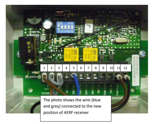
The dip switch of the receiver has to be changed to the follow position:
