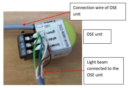
The light beam will connected to the OSE unit. (Photo) The color code of the wires is written to the OSE unit.
