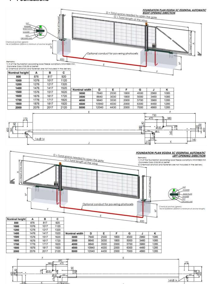
1. Install the ground fixations of the guiding and end post according to the positions indicated on the foundation plan. Therefore following fixation material is required: Chemical anchors M12x160 (minimum 80mm above Finished Ground Level. For anchor depth check installation manual of supplier chemical resin).
